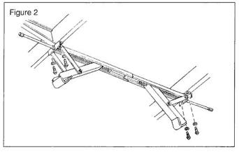
STEP 2. With the stabilizer in the desired location, use the mounting plates as a template. Mark the mounting hole locations on the trailer frame with a center punch. Drill (2 each) 9/32" holes into the trailer frame at each end of the stabilizer assembly corresponding to the holes in the mounting plates (Figure 2).
