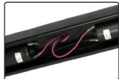
Stabilizer Jack Motor Wires
