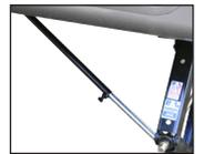
Helps eliminate unwanted movement in your trailer by adding support from the jack's foot to the trailer frame.
