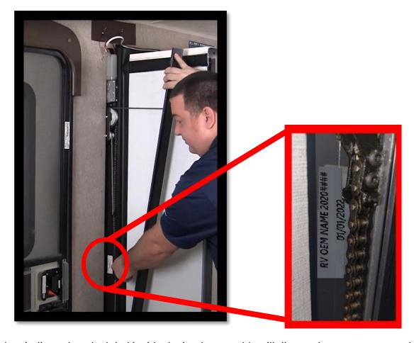
The date indicated on the label inside the jamb assembly will dictate the motor part numbers.
