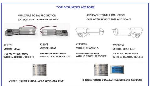
LEFT AND RIGHT ARE DETERMINED BY STANDING INSIDE THE RV FACING THE SLIDE ROOM
