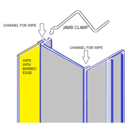
CHANNEL IS PINCHED AT TOP AND BOTTOM TO SECURE THE WIPE SEAL
