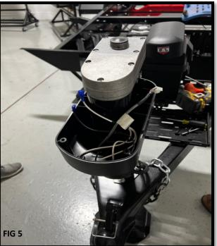
FIG 6. Using a 1/2" wrench or socket, remove the two bolts that hold the motor in place and set the motor aside.
