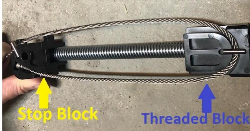
7. Place the threaded block with cable attached into the channel opening and slide it towards the drive end of the channel. Push the threaded block as far down the channel as possible keeping the cable in the correct routing location. Be sure to hold onto the end of the cable and not let it slip into the channel where it cannot be reached.
