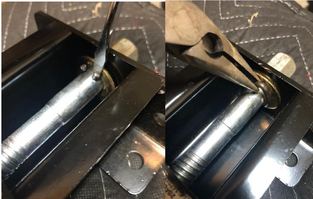
3. If the female threaded block is damaged, you should now be able to slide the threaded rod out of the carrier channel. Please note the position of the flat washers. If the threaded rod block is still attached, use a 3/4" wrench or socket to unthread the rod from the block.
