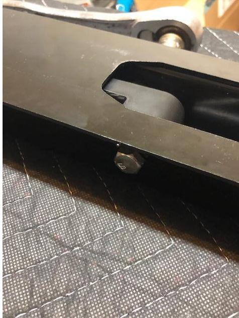
**Step 11:** Continue to crank the threaded rod clockwise until the drive nut and exterior washer is positioned against the channel. **DO NOT OVERTIGHTEN.** Rotate the threaded rod to a position that the retaining pin can be inserted in the hole in the rod and reinstall by tapping lightly back into position. Make sure the washers are in the correct location.
