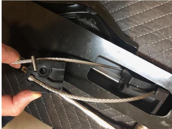
6. Using the new threaded block and the stop block, replace the cable by routing it as noted in steps above. Use the image below as a reference. The cable reinstalls against the channel wall and NOT pointing 'up'.
