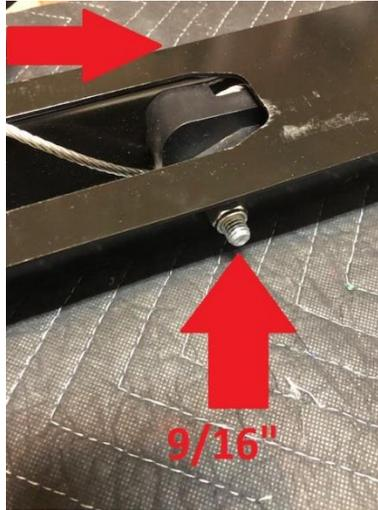
5. Using the cable, pull the threaded block towards the channel opening until it can be removed from the channel. If the threaded block is intact, note the routing of the cable on both blocks for reference during reassembly. Remove the cable & discard the block if damaged.
