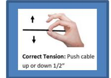
1. Tension the **OUT BTM** cables until the bottom interior standoff brackets contact jamb.
