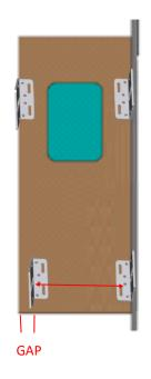
IF THE BRACKETS ARE MOUNTED TO FAR FROM THE EDGE OF THE END WALL ON THE SLIDE, THE CABLES CAN BE TOO LONG TO ADJUST PROPERLY.
