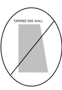
TAPERED END WALLS ARE ONLY APPLICABLE ON THROUGH FRAME SLIDES
